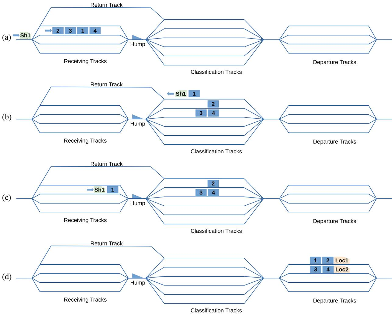
FIGURE 5 Example: multi-stage classification with cars ordering
