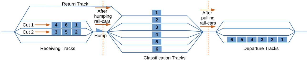
FIGURE 10 Three main steps of the sorting-by-block algorithm
